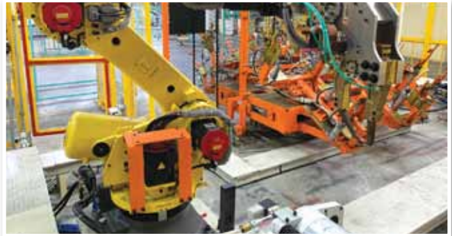
Spot Welding – Body Side Sub
